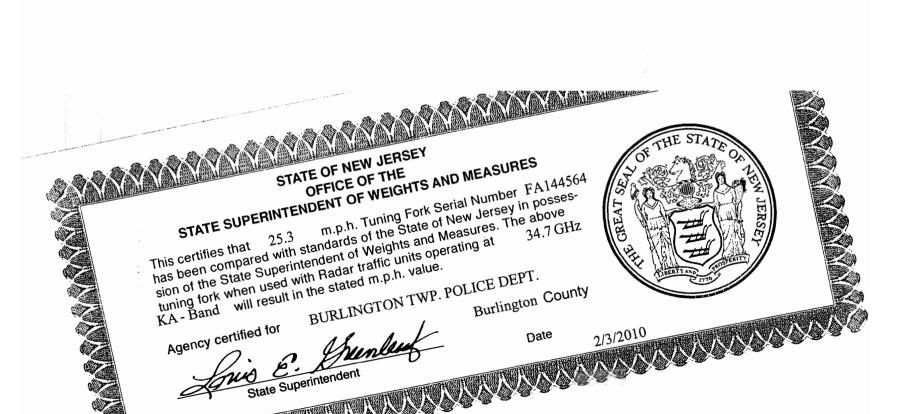
This certifies that 25.3 m.p.h. Tuning Fork Serial Number FA144507 has been compared with standards of the State of New Jersey in possession of the State Superintendent of Weights and Measures. The above tuning fork when used with Radar traffic units operating at 34.7 GHz KA-Band will result in the stated m.p.h. value.
