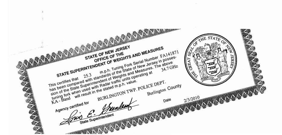
This certifies that 25.3 m.p.h. Tuning Fork Serial Number FA144511 has been compared with standards of the State of New Jersey in possession of the State Superintendent of Weights and Measures. The above tuning fork when used with Radar traffic units operating at 34.7 GHz KA - Band will result in the stated m.p.h. value.
