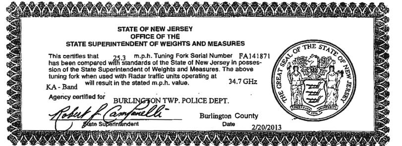
m.p.h. Tuning Fork Serial Number This certifies that has been compared with standards of the State of New Jersey in Bostes 871 sion of the State Superintendent of Weights and Measures. The above tuning fork when used with Radar traffic units operating at 34.7 GHz will result in the stated m.p.h. value.
