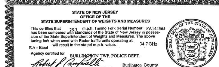
This certifies that 25.3 m.p.h. Tuning Fork Serial Number has been compared with standards of the State of New Jersey In Foetal 565 sion of the State Superintendent of Weights and Measures. The above tuning fork when used with Radar traffic units operating at 34.7 GHz will result in the stated m.p.h. value.
