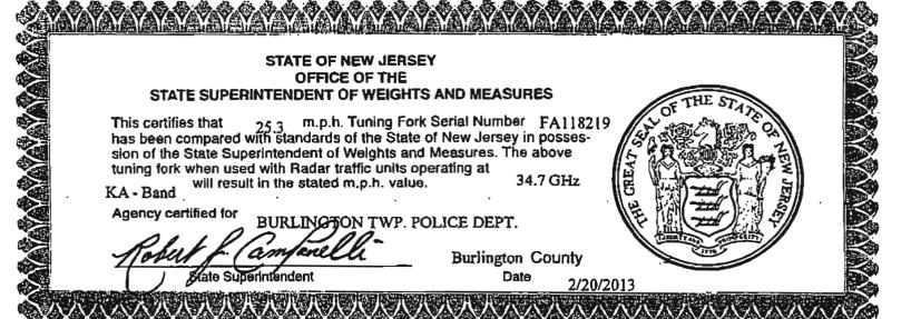
m.p.h. Tuning Fork Serial Number This certifies that has been compared with standards of the State of New Jersey in Books 219 sion of the State Superintendent of Weights and Measures. The above tuning fork when used with Radar traffic units operating at 34.7 GHz will result in the stated m.p.h. value.
