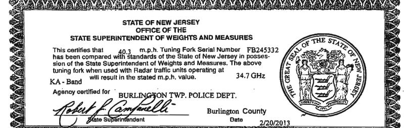
This certifles that 40.3 m.p.h. Tuning Fork Serial Number has been compared with standards of the State of New Jersey in possess 132 sion of the State Superintendent of Weights and Measures. The above tuning fork when used with Radar traffic units operating at will result in the stated m.p.h. value. 34.7 GHz
