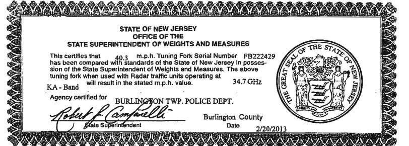
This certifies that 40.3 m.p.h. Tuning Fork Serial Number has been compared with standards of the State of New Jersey In passas 29 sion of the State Superintendent of Weights and Measures. The above tuning fork when used with Radar traffic units operating at will result in the stated m.p.h. value. 34.7 GHz
