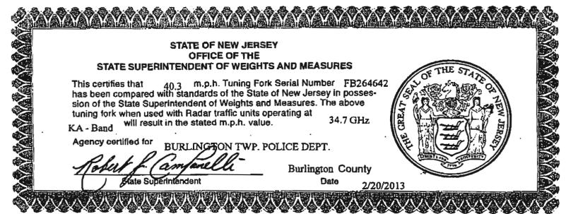
This certifies that m.p.h. Tuning Fork Serial Number This certifies that 40.3 m.p.h. Tuning Fork Serial Number has been compared with standards of the State of New Jersey in 5034642 sion of the State Superintendent of Weights and Measures. The above tuning fork when used with Radar traffic units operating at 34.7 GHz will result in the stated m.p.h. value.
