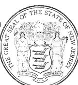
FB276763 40.25 m.p.h. Tuning Fork Serial Number This certifies that has been compared with standards of the State of New Jersey in possession of the State Superintendent of Weights and Measures. The above tuning fork when used with Radar traffic units operating at 34.7 GHz KA - Band will result in the stated m.p.h. value.
