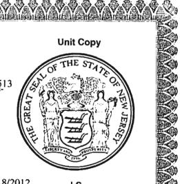
m.p.h. Tuning Fork Serial Number FA134588 This certifies that 25.3 m.p.h. Tuning Fork Serial Number FA13458 has been compared with standards of the State of New Jersey in possession of the State Superintendent of Weights and Measures. The above tuning fork when used with Radar traffic units operating at 34.7 GHz will result in the stated m.p.h. value.
